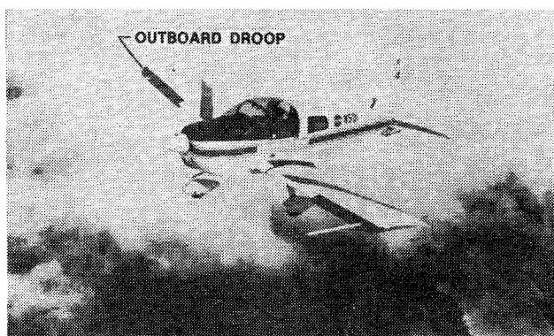
Fig. 1 Test airplane with baseline outboard leading-edge droop.
